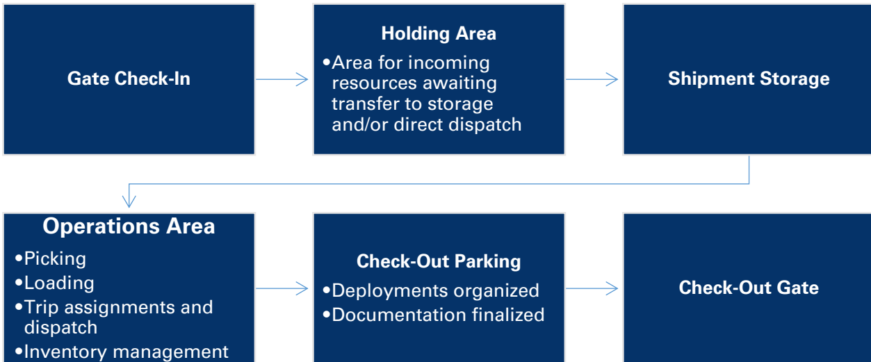
Figure 5: Staging Area Process Diagram, such as for Incoming and Out-going Vehicle Movements that Support Receipt, Storage, and Shipping of Commodities as Part of a CPOD Operation
